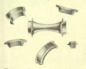
The cups and cones used in the construcion of Hyslop Bicycles are specially heatreated. They are case hardened only on uch surfaces as receive the direct wear, to a ufficient depth to hold the load. (See illusration.) This gives the proper wearing surace for the balls, but tends to remove all orittleness from the other parts. Hyslop Frame Reinforcements in Sections
