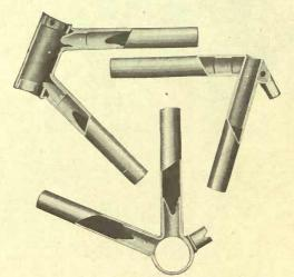
This cut shows the great strength of the improved reinforced joint construction of the Hyslop frame. The dip-brazing method makes for perfect amalgamation throughout the joint and entire length of the reinforcement. Every part carefully tested before being assembled.
