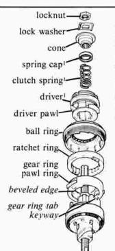
Install ball ring. Push pawls in and rotate ring until seated over pawls. Install driver.1 Push pawls in and turn driver clockwise until it seats in ball ring. Install spring and spring cap. Install cone, lockwasher and locknut. Adjust bearing. If bearing runs rough, check spring cap.1
