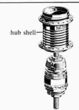
Position hub shell long end up and lower over assembly until it seats.
