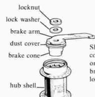
Slip hub shell over assembly. Rotate counter-clockwise until shell race seats on large retainer. Install brake cone, brake arm (brand name facing out) and locknut. Adjust bearing.
