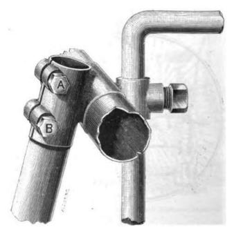
FIG. 42.-JOINT FOR CONVERTING A TANDEM INTO A SINGLE MACHINE.
