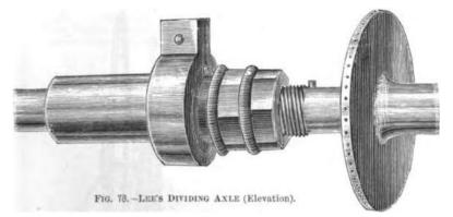
dividing sleeve occupies but a small space (see Fig. 78). The safety tail at the back prevents the machine from falling when the wheel is taken off. In fact, Lee's patent may be justly termed one of the simplest and most effective "folders" of the day. It can be applied to most machines at small cost.
