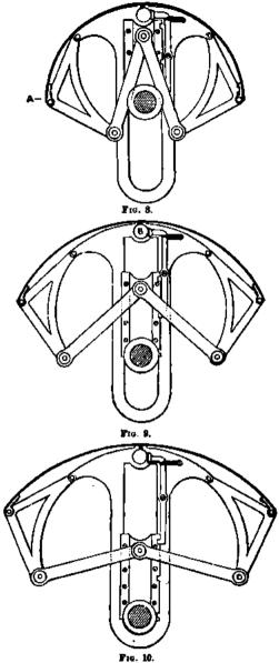
SIDE ELEVATIONS OF SEGMENTS AT DIFFERENT POWERS.
