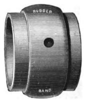
FIG. 42-FRONT WHEEL BEARING BOX, WITH RUBBER CUSHION DETACHED FROM FORK.
