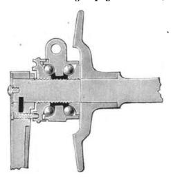
FIG. 6.-THE CHALLENGE FRONT WHEEL BEARINGS (Soctional View).
