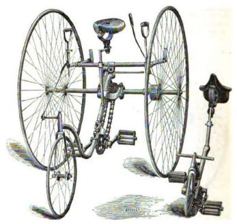
FIG. 5.-THE EXCELSION CONVERTIBLE REVERSIBLE TANDEM ROADSTER (Single Form, Front Steerer).
