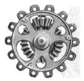
FIG. 39.-INTERIOR OF STARLET'S GRAB, ONE BRYELLED WHERL REMOVED.
