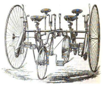
FIG. 43.-THE DOUBLE TANDEM CONVERTIBLE FOUR-IN-HAND BOADSTER.
