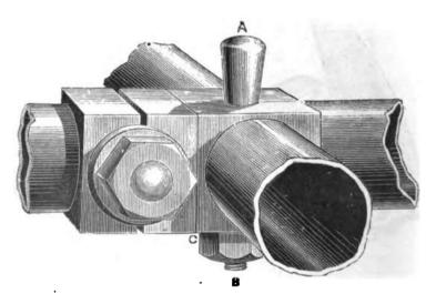
FIG. 38.-DETACHING BOLT OF COVENTRY CONVERTIBLE HOADSTER.
