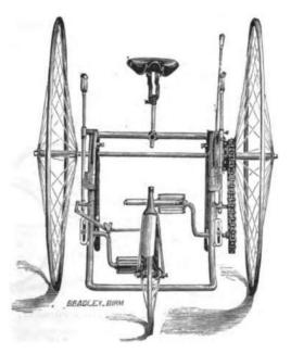
FIG. 32.-THE REVERSIBLE CENTAUR TANDEM HOADSTER (converted into a Single).
