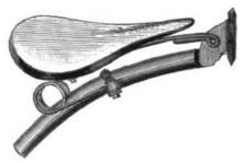
FIG. 23.—HARRINGTON'S SPECIAL ADJUSTABLE TRICYCLE SPRING.
