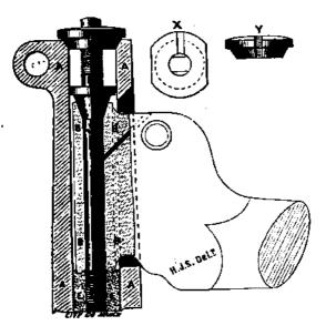
FIG. 39,-THE RUCKER HEAD (Swindley's Patent).
