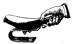
FIG. 29 .-- WITHDRAWING SADDLE.
