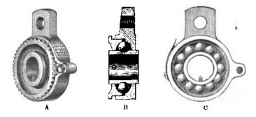
FIG. 19.-BOWN'S BALL BEARINGS FOR CRANK SHAFT.
