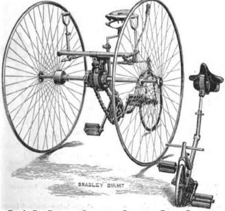
FIG. 4.-THE EXCELSIOR CONVERTIBLE REVERSIBLE TANDEM ROADSTER (Single Form, Rear Stoerer).
