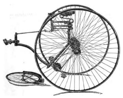
FIG. 25.-THE LADIER' CUMARD NO. 3 ROADSTER (With pilot wheel removed, showing Tandam connecting joint).
