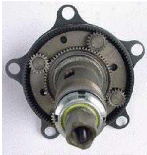
Schlumpf epicyclic internals (huge sun gear) and heel shifter 14
