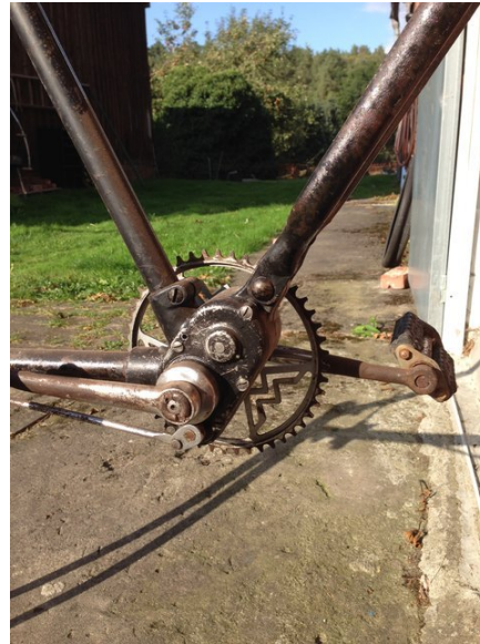
1936 Wanderer original 2 speed with shift rod
