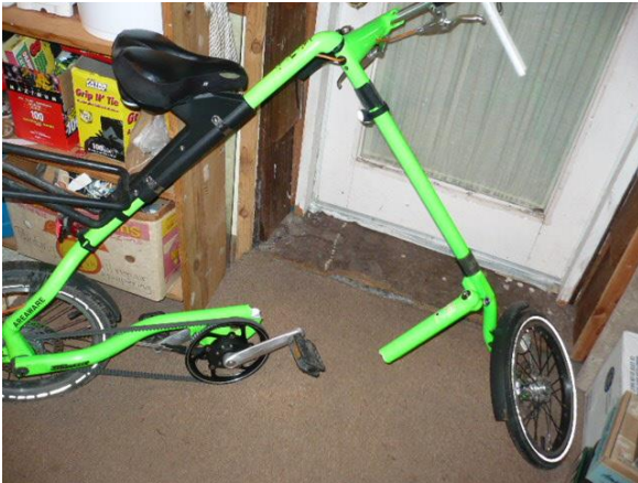
The author's Schlumpf 2 speed Strida, after frame weld failure
