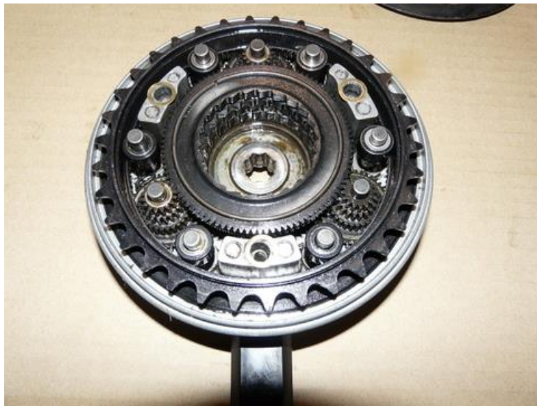
Inside the complex FM-5 crankwheel (Shimano FG-5S10) - huge sun gear for high ratios
