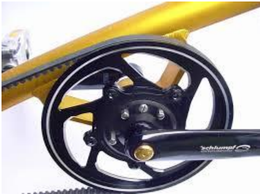
Strida version of the Schlumpf, note golden shift button
