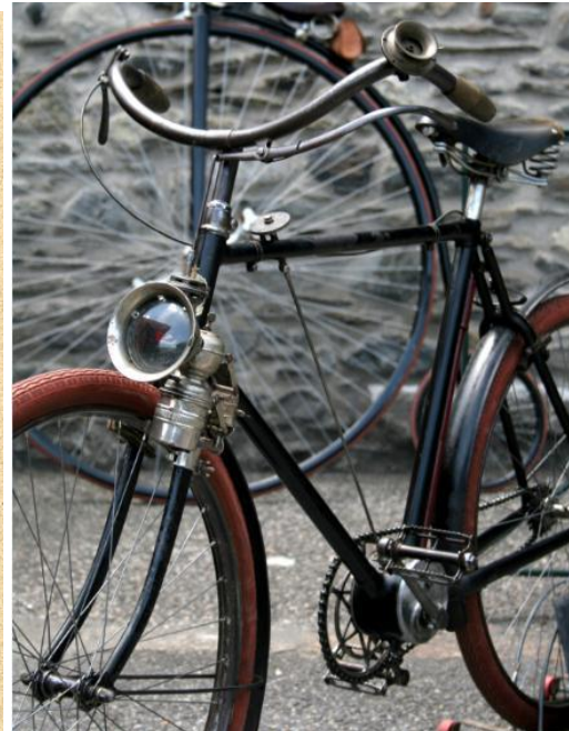
The Magnat-Debon 3 speed gearbox (Direct High 1, Normal 2, Low 3) An Edwardian Magnat-Debon, note rotating disc on x-bar 19
