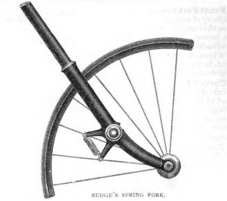
spiral spring. As a result, all the weight placed on the forks is borne by the springs, which give to every obstacle.
