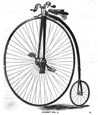
both wheels. Hollow front and back forks. Stanley head, 4 in. centres. Pear-shaped horn handles, 28in. cowhorn bars. 18in. 16 W.G. weldless steel backbone. Humber scroll spring. L.D. suspension saddle. Adjustable saw step. D.L.S. brake. Leg-guard. Valise, spanners, oilcan, lamp and bell. Weight 35lbs.
