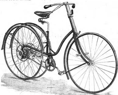
and revolve together as one. The object of this arrangement is to permit of the machine standing by itself for mounting, dismounting, or sitting still—of course when on a level road.
