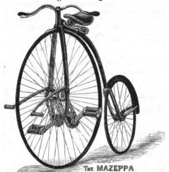
like ordinary bicycle. Forks zin. behind bearings. Hollow front and semi hollow back forks. Stanley head, 4in. centres. Pear-shaped horn han dles, 28in cowhorn bars. Weldless steel backbone. Arab cradle spring. L.D. suspension saddle. Circular step. D.L.S. brake. Leg-guard. Valise, spanners, oilcan, lamp, and bell. Weight 40lbs.
